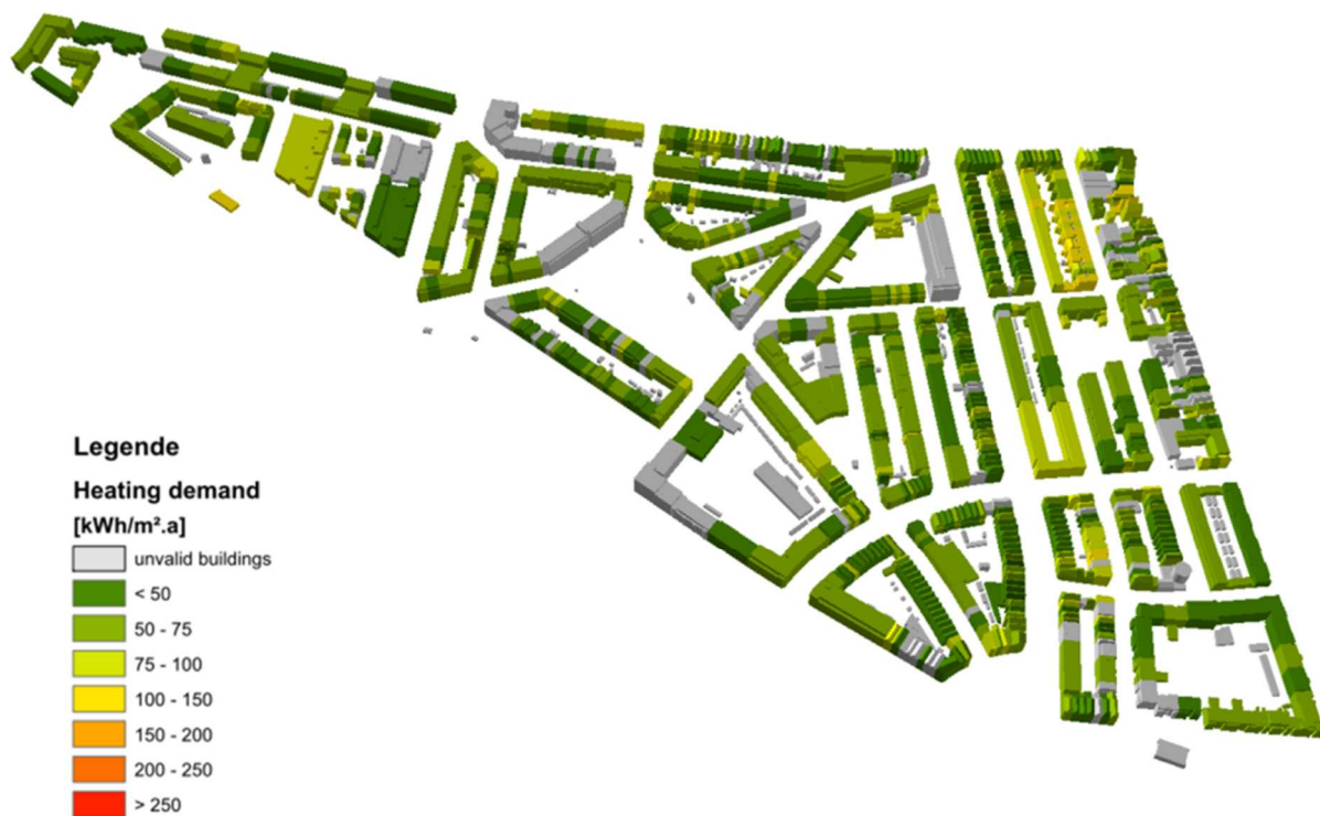
Fig. 33: Specific heating demand mapping – Bospolder scenario refurbishment
