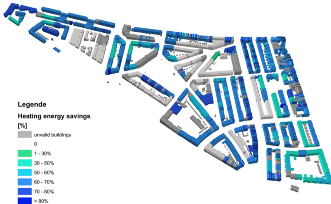
Fig. 35: Heating savings potential mapping – Bospolder scenario refurbishment
